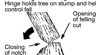
**NOTE:** Before felling cut is complete, use wedges to open the cut when necessary to control the direction of fall. To avoid kickback or chain damage, use wood or plastic wedges, but never steel or iron wedges.
