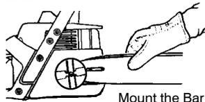
6. Carefully remove the chain from the package. Hold chain with the drive links as shown.
