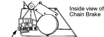
4. Turn the adjusting screw by hand counterclockwise until the adjusting pin just touches the stop. This should allow the pin to be near the correct position.
