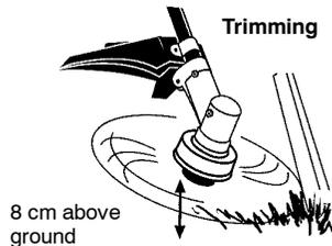
**SCALPING** - The scalping technique removes unwanted vegetation. Hold the bottom of the trimmer head about 8 cm above the ground and at an angle. Allow the tip of the line to strike the ground around trees, posts, monuments, etc. This technique increases line wear.
