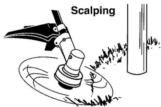
**MOWING** - Your trimmer is ideal for mowing in places conventional lawn mowers cannot reach. In the mowing position, keep the line parallel to the ground. Avoid pressing the head into the ground as this can scalp the ground and damage the tool.
