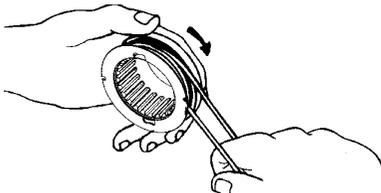
7. With your finger between the lines, wrap the lines evenly and firmly around the spool in a clockwise direction.
