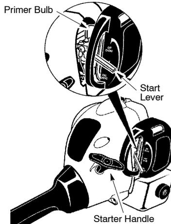
5. Pull starter rope handle sharply until engine starts and runs.
